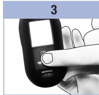
Put the battery door back in place and snap it closed.
