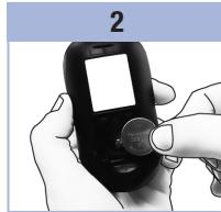
Remove the old battery. Insert the new battery with the **(+)** side facing up.
