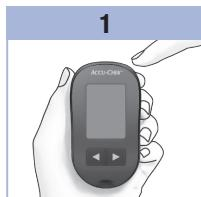
Press and release ① to turn the meter on.
