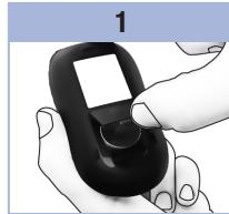
Open the battery door on the back of the meter by pushing the tab in the direction of the arrow and pulling the door up.
