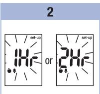
Press and release ① repeatedly until **set-up** and the flashing **1Hr** or **2Hr** appear on the display.
